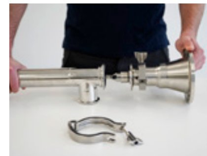
Remove pump tube
