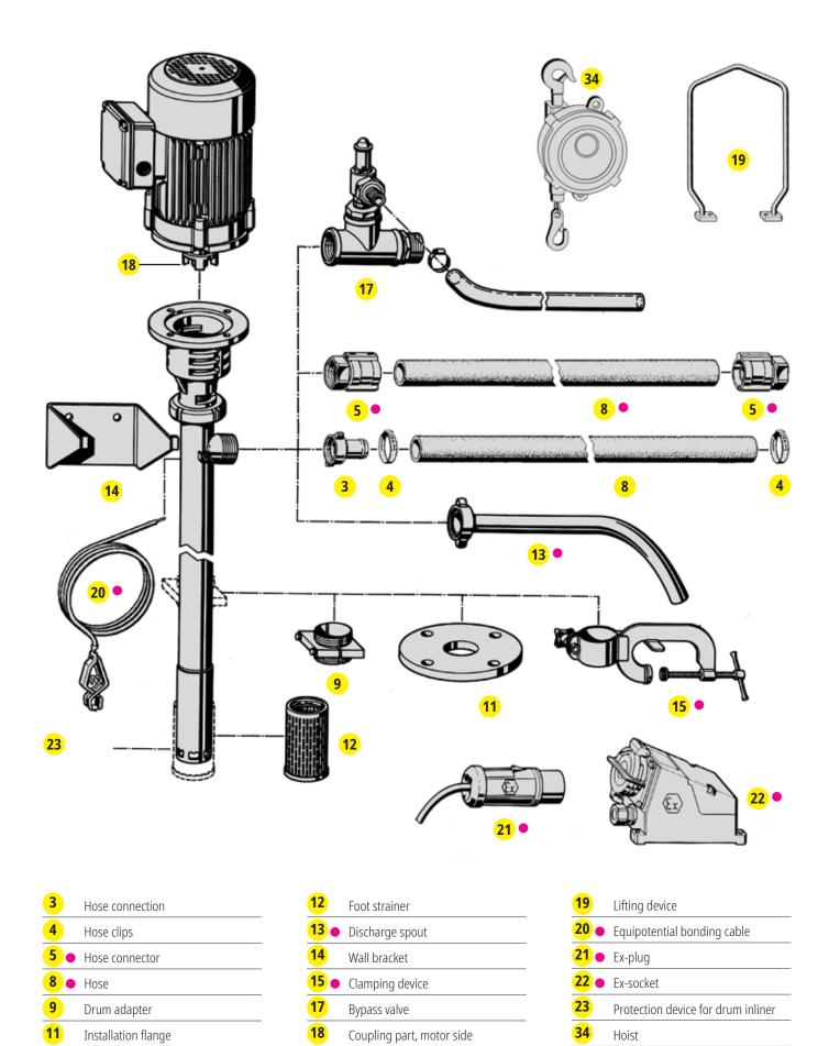
Suitable for transferring combustible and easy inflammable liquids (e.g. ethanol, petrol) or in explosive hazard area.
